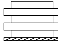
Profile C Severe Puncture Hazard
